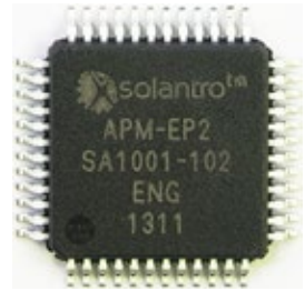
Complete analog front-end for DC-DC power conversion
