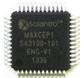
Microcontroller for managing real-time power converters
