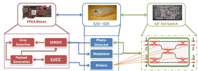
Fig. 1: Controlled SiP switch system setup overview.
