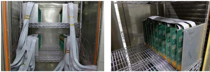
Figure 7: Card set up in thermal cycling chamber
