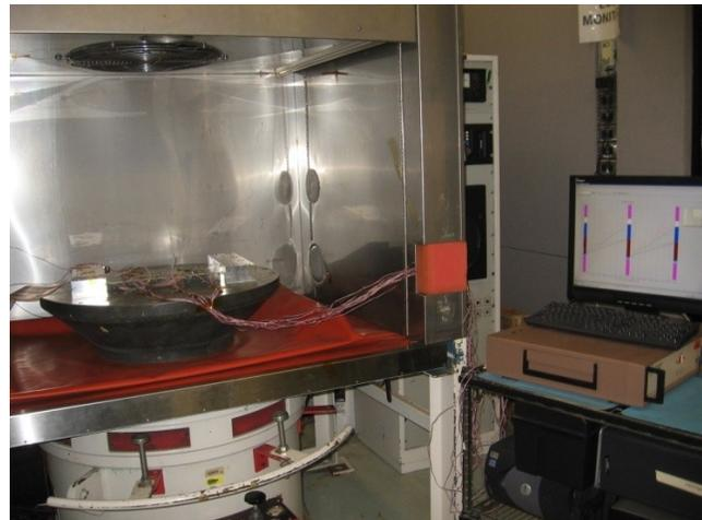
**Figure 3: Thermal test chamber & vibration table**
