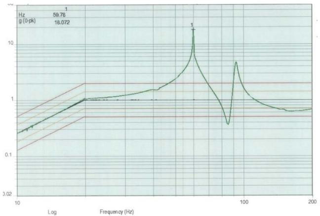
**Figure 5:** T3-50 Sine 1 Gpk 4 Oct/min at 125<sup>°C</sup>
