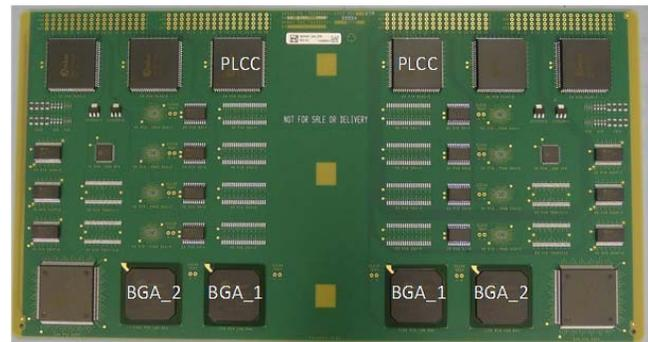
**Figure 1:** Test vehicle & tech types
