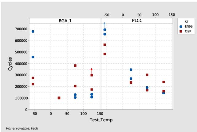
**Figure 8:** Cycles to Failure Vs. Test temperature
